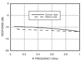
Unless otherwise noted, all measurements performed as a downconverter, with low side LO & IF = 200 MHz.
